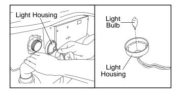
To replace the light bulb, pull the old bulb out of the housing and insert a new bulb. Re-attach the light housing to the spa shell. Re-attach the access cover to the spa.
